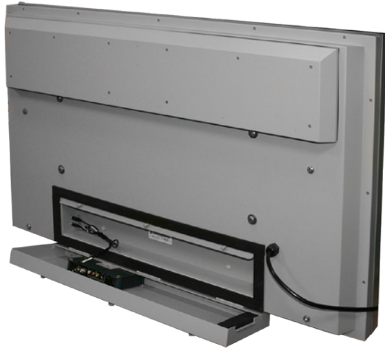
Internal Media Compartment shown with Cisco Digital Media Player
